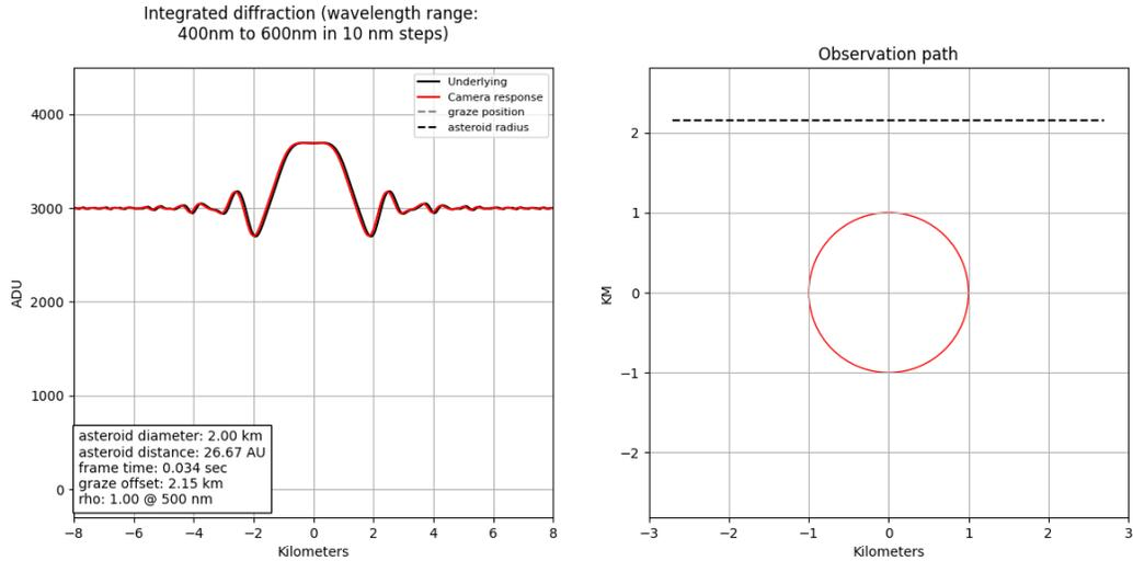
The luckier observer of this event might have been on the centerline of the occultation path and would have had to use the model light curve shown below to extract the chord position and duration from his recording:
