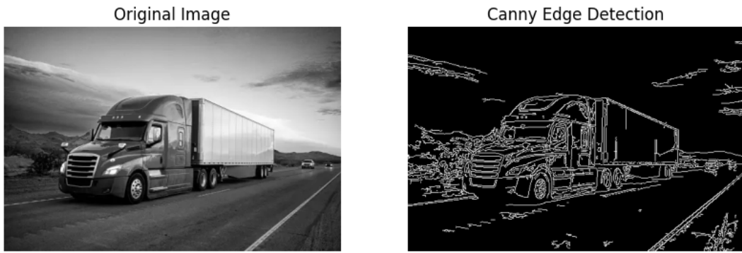
Figure 4: An image before and after applying the Canny filter for edge detection.
