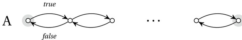
**Figure 11-3.** A single “row,” representing the variable  $A$  the Boolean expression we’re trying to satisfy. If the cycle passes through from left to right, the variable is true; otherwise, it’s false
